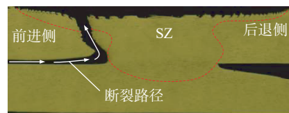
图9 转速1504 r/min、焊速207 mm/min、下压量0.12 mm参数下的接头断裂路径 Fig.9 Joint fracture path under the parameters of 1504 r/min rotating speed, 207 mm/min welding speed and 0.12 mm plunge depth
